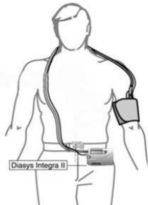
Figure 1: The image above shows how the monitor is set up on your body. The cuff will be wrapped around your arm and a lead will connect this to the monitor, which sits in a pouch on the waist belt.
